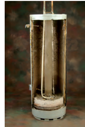
Scaled Water Heater.tif
